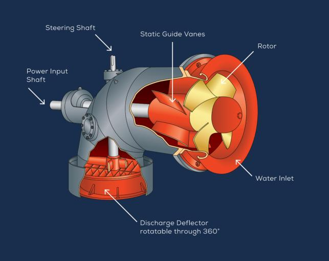
Our Tees White Gill cross shaft thruster (CS) has a static thrust from 1003kgs to 6974kgs, and as our most compact design, is an excellent choice for retrofit applications, or those with limited spaces - such as canal or river barges.
